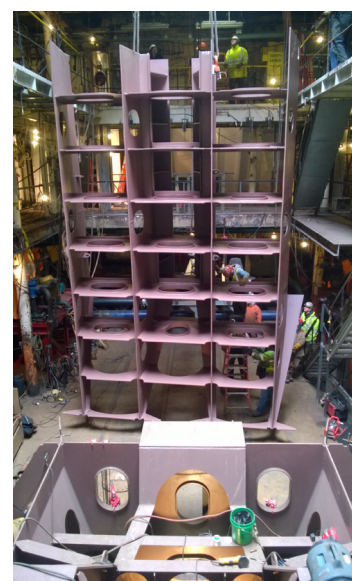
On this massive foundation now rests the JACKSON's new engine. Photo courtesy Fraser Shipyards, Inc.
