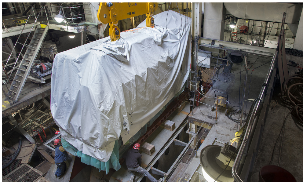
The MUNSON's new engine is carefully lowered into place. Photo by Chris Winters.
