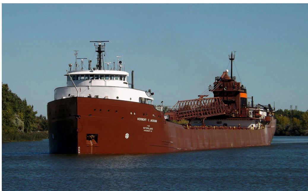
Repowering of the HERBERT C. JACKSON completes Interlake Steamship's conversion of its steamships to internal combustion engines. Photo courtesy The Interlake Steamship Company.
