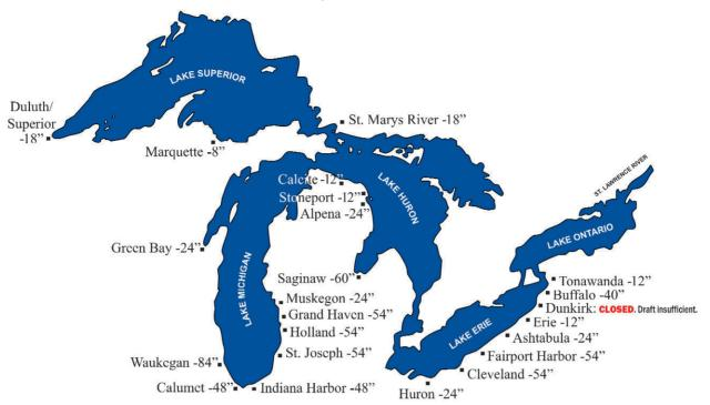
Commercial vessels working the Great Lakes are leaving behind cargo virtually every time they load because of inadequate dredging of deep-draft ports and waterways. The map above uses select Great Lakes ports to illustrate how many inches of loaded draft the dredging crisis is costing the industry. Graphic courtesy U.S. Maritime Administration.
